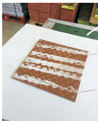
Step 4: Wrap the wire around tiles and twist at other edge.
