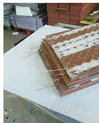
Step 5: Make a stack of tiles wrapped in wire.
